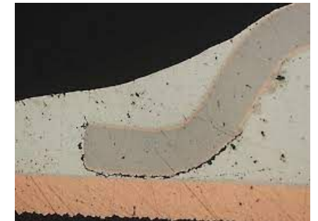
Solder Pad Structural Failure in various package types
